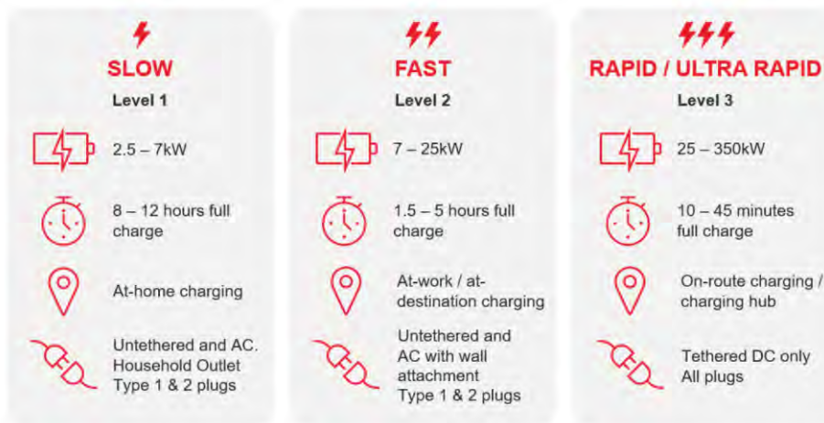
Figure 2 – EV charging levels
