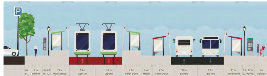
Prominent side platform TT/ LRT station cross-section (Murdoch Station, 2)
