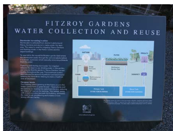
The underground storage tank, constructed wetland and water transfer pumping and storage system at Fitzroy Gardens ensures that the water quality is maintained for irrigation purposes
