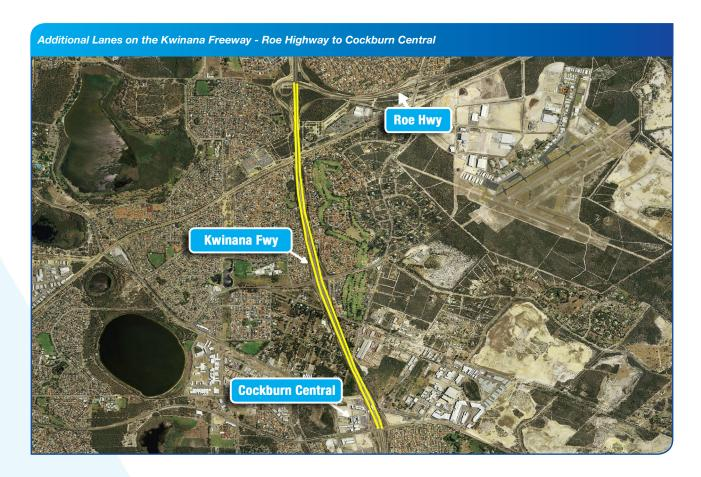
Estimates for the additional lanes are likely to cost in the order of \$40 million, which includes the relocation of services and the extension and structural reinforcement of the freight rail bridge just south of Roe Highway to accommodate the additional width.
